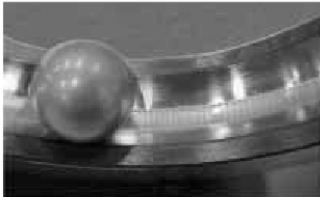
Figure 1: Bearing currents can cause "bearing fluting", a rhythmic pattern on the bearing's races.
